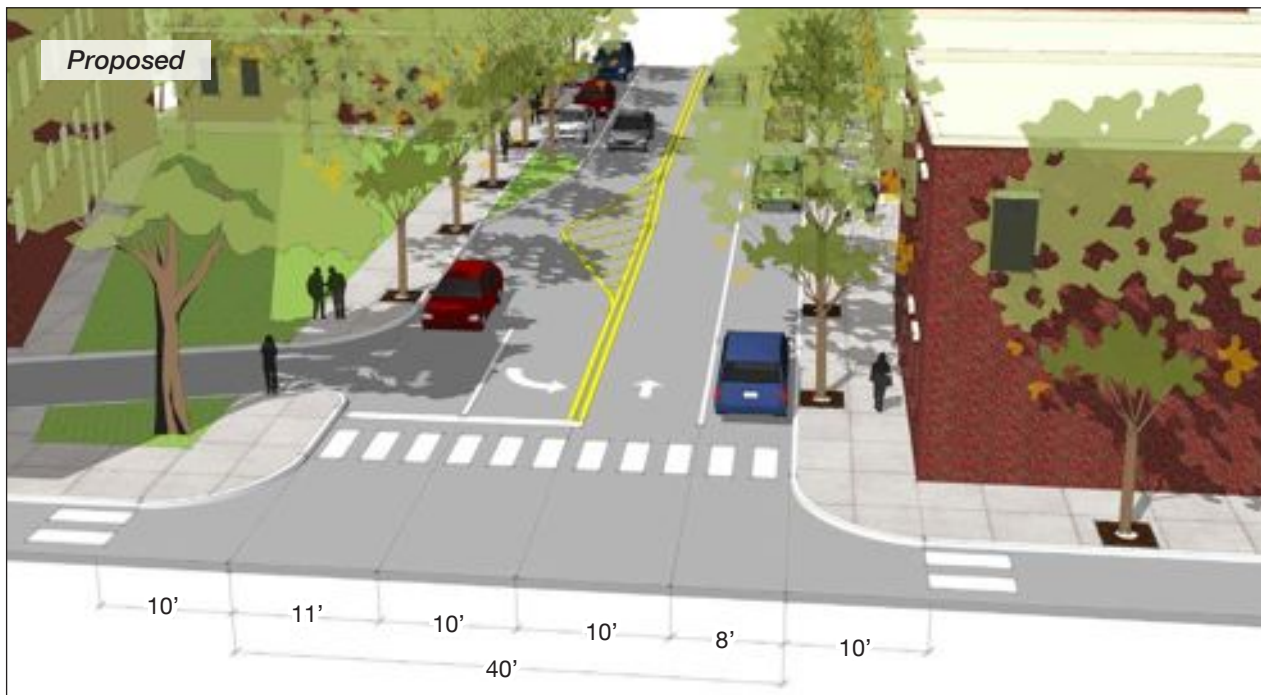
The slip-lane entry into the Roy garage requires reconfiguration as Market becomes two-way. Pains should be taken to preserve the existing tree.
